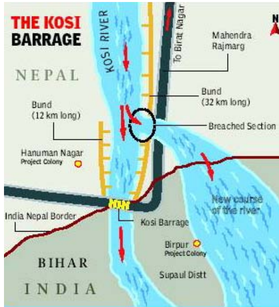
Kosi Embankment Breach.
